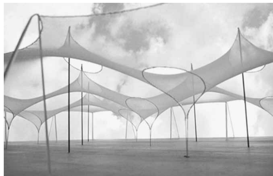
Form-finding study for the support of textile membranes and rope nets
